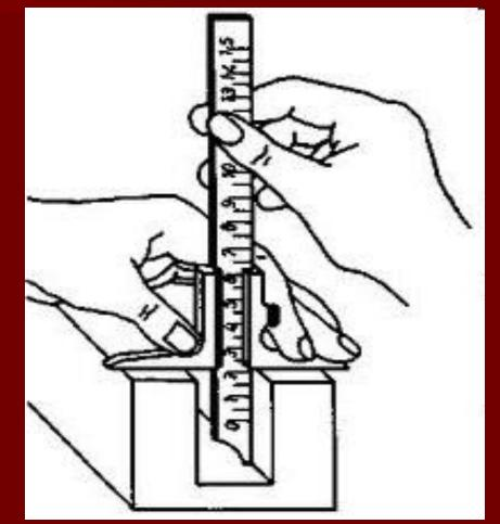
While using this instrument the base is held over the reference surface and lower beam go downward until it contact the bottom surface of the hole.
