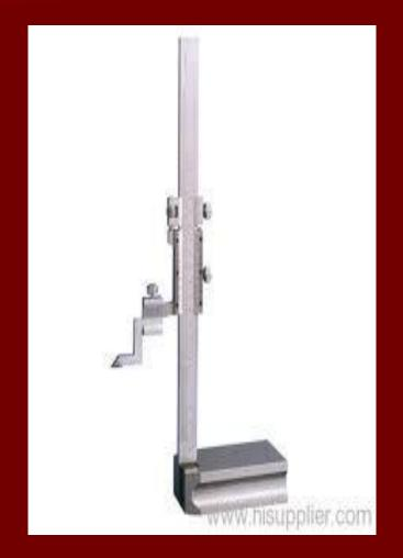
The vernier height gauge is design for the accurate measurement and marking of vertical height above the surface plate.
