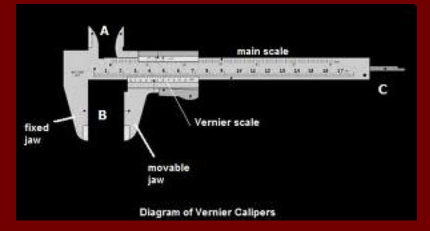
Vernier calliper reading = main sacle reading + The number of division which exactly coincide with a number of main division x Least count
